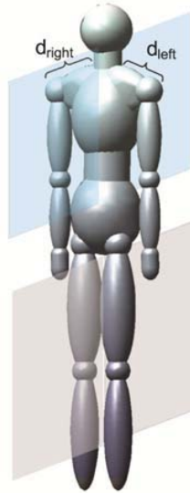
Figure 5.4. Symmetry planes fitted to the upper and lower half of the body. Corresponding distances d_{left} and d_{right} were averaged to make the body geometry laterally perfectly symmetric.
