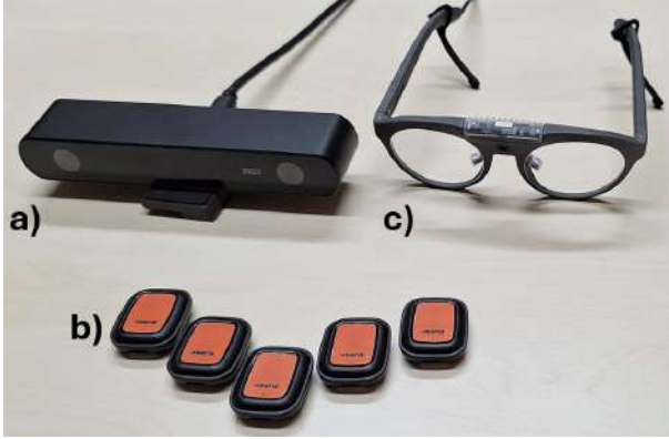
Fig. 2: The used sensor modalities to collect various data. a) ZED2i stereo camera b) Movella DOT IMUs c) Eye tracking system Pupil Labs Neon.
