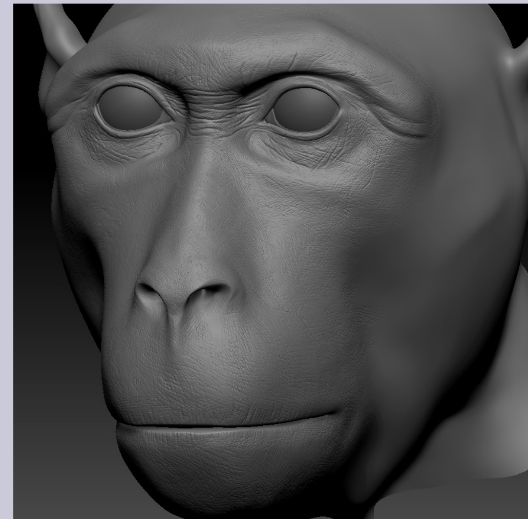
Figure 3: Refined surface (7.3 million polygons) created in Autodesk Mudbox to extract high frequency details for low resolution mesh.
