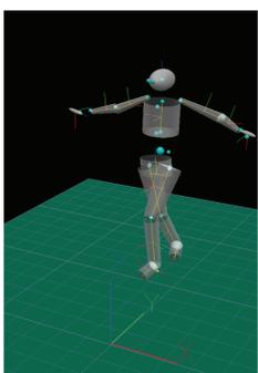
Motion of 15-segment rigid body model was fit to the 3D motion capture data
