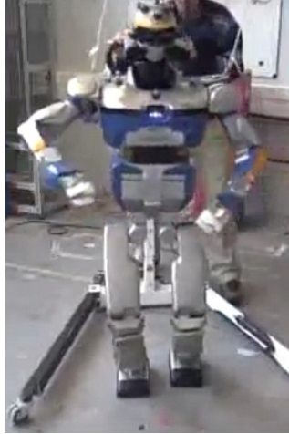
Fig. 10 Real HRP-2 robot performing walking-reaching sequences at LAAS-CNRS.
