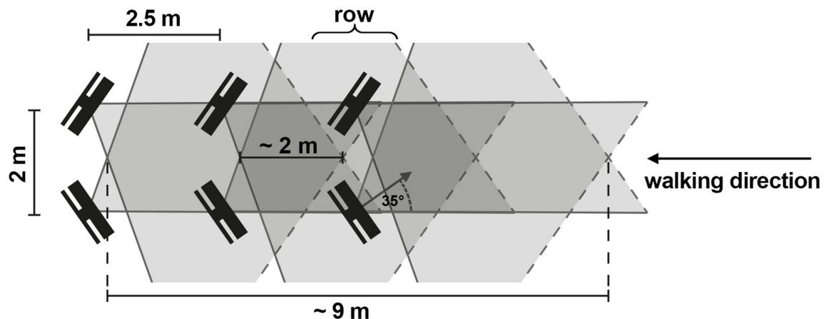
**Fig 4. Arrangement of the Kinect sensors illustrating the overlapping tracking volumes.** Sensors were arranged using this pattern but then spatially calibrated to achieve high precision. The theoretical length of the tracking volume in walking direction using this setup is about 9 meters. The Kinect sensors were arranged in a way ensuring that the VICON tracking volume was completely covered.
