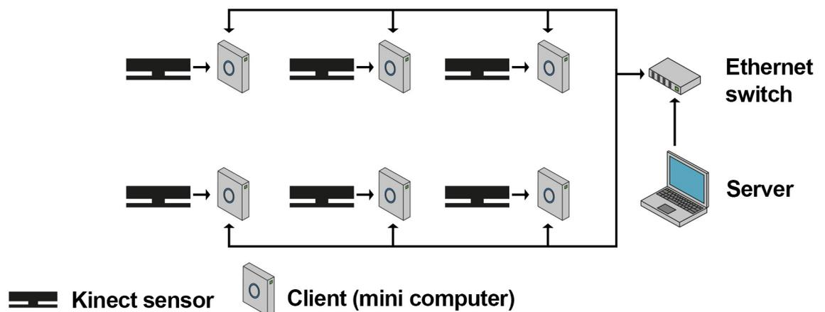
**Fig 1. Architecture.** Connections between the Kinect sensors, Zotac mini computers running the client software and the server computer in a setup with six Kinect sensors.
