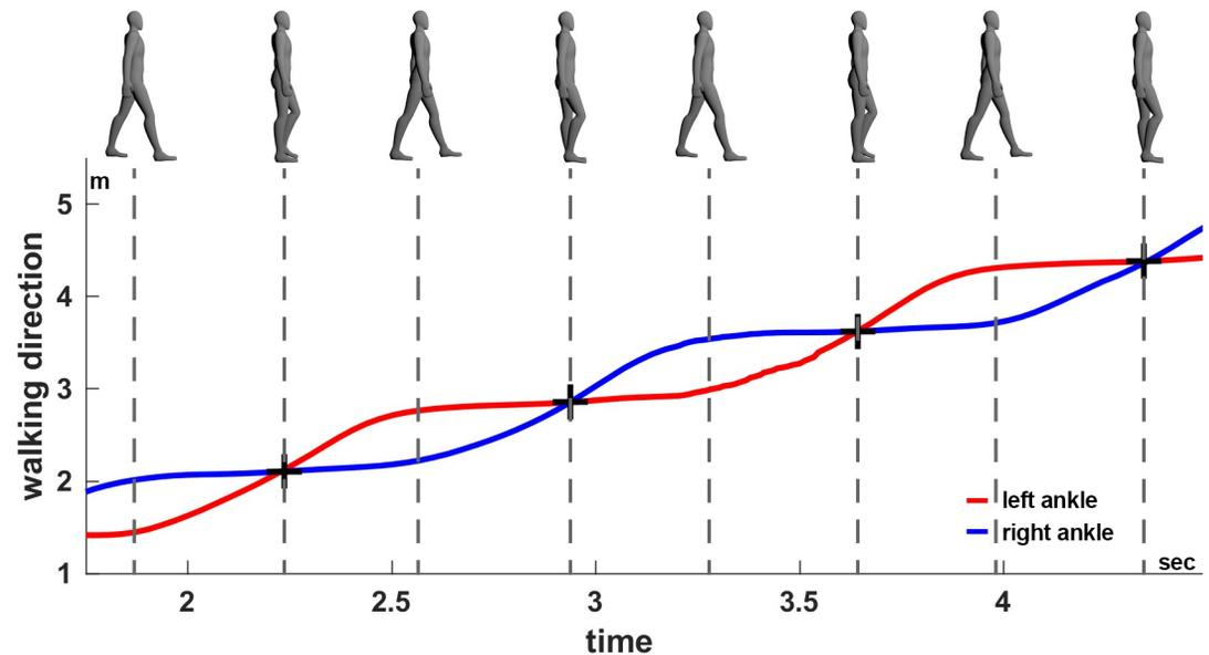
**Fig 7. Identification of the foot events.** Foot events (black crosses) based on the ankle trajectories, here exemplified using the Kinect skeleton averaged across all sensors. Using the same procedure foot events were extracted from the VICON data. Top: Snapshots of the body posture during walking, bottom: ankle position of the left (red) and right (blue) foot in walking direction.
