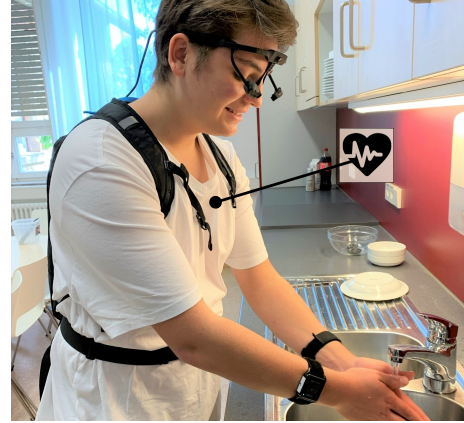
Fig. 2. Equipment as worn by the patients. Sensors include an eye tracking device, an ECG chest belt, and inertial sensors on each wrist. Additionally, participants carried a backpack with a tablet for data collection.
